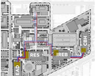
Proposed east campus loop Existing / Proposed Chilled Water Lines Existing / Proposed Hot Water Lines Distributed Infrastructure Locations
